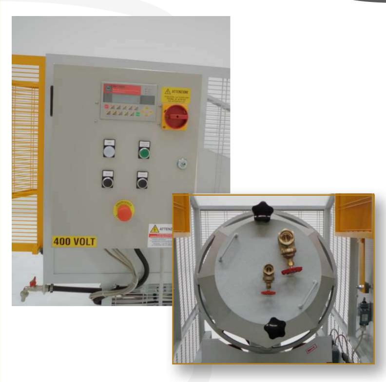
Buratto RB machines are available with electronic speed control and extending the code PMP. Standard cover is provided with an exhaust filter and endowed with screw polymer cap. To fix the cover to the barrel, it is equipped with two screws. It is recommendable, for wet processes, to foresee (at customer charge) a grid on the floor for drainage of wastewater.
