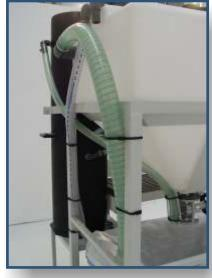
On the upper part of the process tank is provided an "overflow" of security, connected with appropriate piping to the filter bag. Also the upper side of the activated carbon column provides an overflow that comes into operation during the periodical phase of counterwashing;
