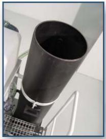
Superior loading side of the column with activated carbon. The column is of «Gravity» type, made of HDPE.
