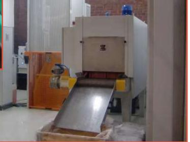
Hot air drying tunnels, with belt and electric heating. The Rollwasch® Drytun range includes stainless steel belts with extra small mesh [XS].
