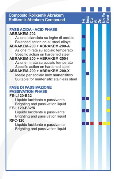
Rollkemik Abrakem is a range surface conversion treatments and superfinishing of high precision components.
