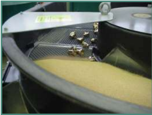
RWO-AS-3/G - unloading phase of dried brass articles
