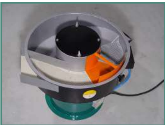
RWO-AS-4-GM/SR - the smallest version, without lining, has a "bridge" removable flap.
