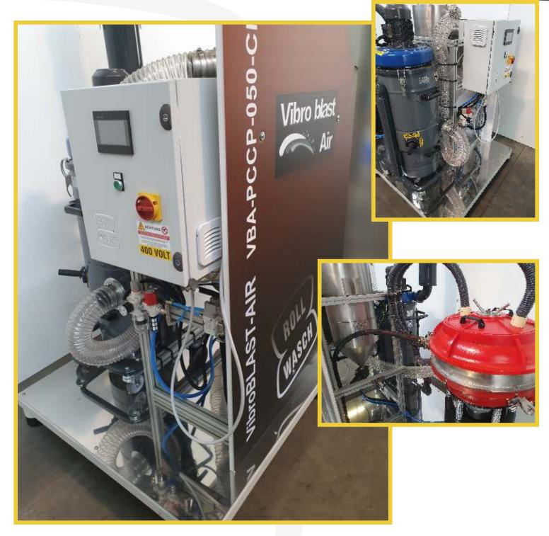
The **VibroBLAST Air DP** line in the above picture with suction filter in ATEX version (expecting certif. within 2021) is designed and manufactured to be supplied on a technological pallet, to make its installation immediate through a simple plug-&-play operation.
