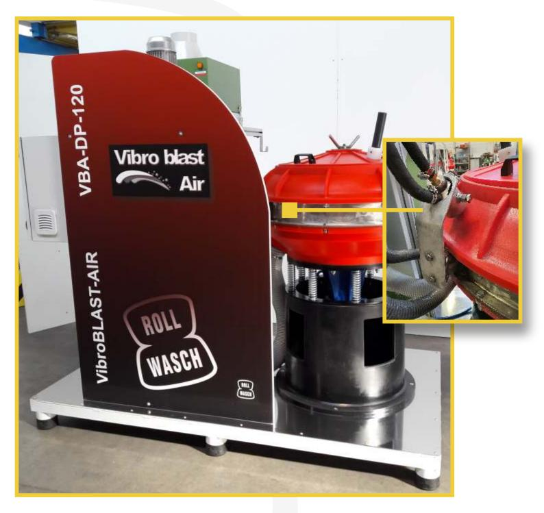
This machine is based on a circular 120-liter-capacity vibrator with tank in PU and lid, a depression sandblasting unit with cyclone and filter cabinet, a control panel with inverter, PLC and touch screen, a sand drain filter on the tank bottom. On the lid of the machine there is an air inlet snorkel, while the blasting nozzle is in the perimeter ring «SN» (acronym of Side Nozzle). Finished pieces can be unloaded from a total unloading door (if they are small) or taken from the top.
