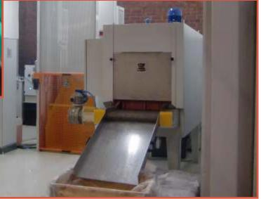
Hot air drying tunnels, with belt and electric heating. The Rollwasch® Drytun range includes stainless steel belts with extra small mesh [XS].
