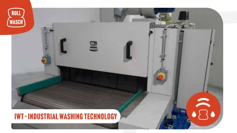
In the Industrial Washing Technology macroarea, Rollwasch® has perfected its own plant vision made of belt conveyor tunnels, water screws or special bi-directional screw drums (RotoROLL).
