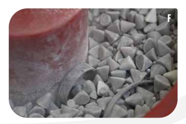
Some typical examples of the so-called «DRY» processes can be: deburring and/or smoothing in self-tumbling - piece against piece (A); deburring and/or smoothing with specific media for dry cycles such as QF or HPM (F); fine smoothing and/or dry polishing with granules impregnated with suitable cremes or pastes (G).
