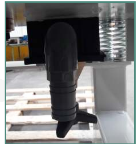
Effluents exhaust valve in PU
