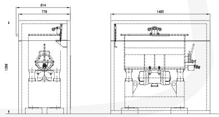
AFOCOP-BOX-150 and AFOCOP-BOX-350 are actioned by 2 gas springs, while AFOCOP-BOX-770 is actioned by PNEUMATIC device.
