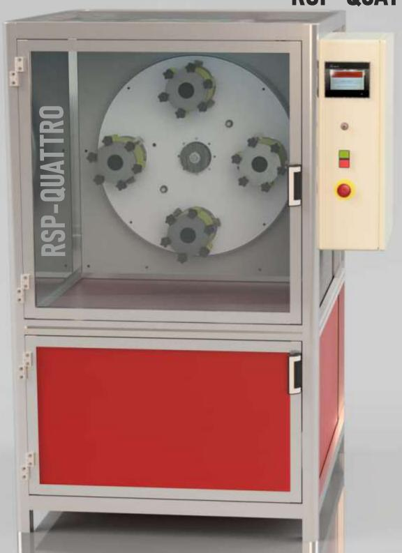
**NEW DESIGN ALSO MEANS FREE CHOICE OF FRAME** i.e.: STANDARD as in the version shown here, complete with compartment and door allows the storing of barrels, abrasives etc., or with final extension **SV** (Simplified, without compartment with door) or, finally: **DT** (Desk Top, table-top) - all equipped with control panel with a 4.7" touch screen panel, plc, inverter, emergency and interlock door closure;
