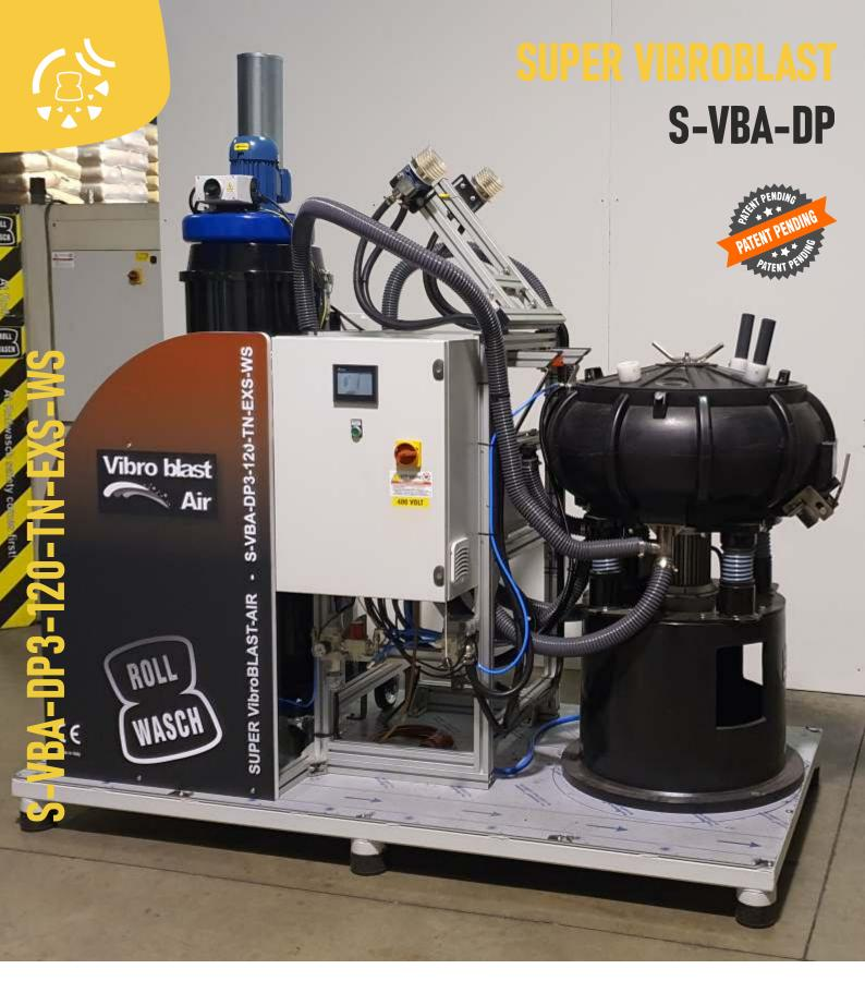
The **Super VibroBLAST Air DP** line is designed and manufactured to be supplied on a technological pallet, to make its installation immediate through a simple **plug-&-play** operation.
